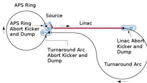
Figure 4: Configuration of a possible abort system.
