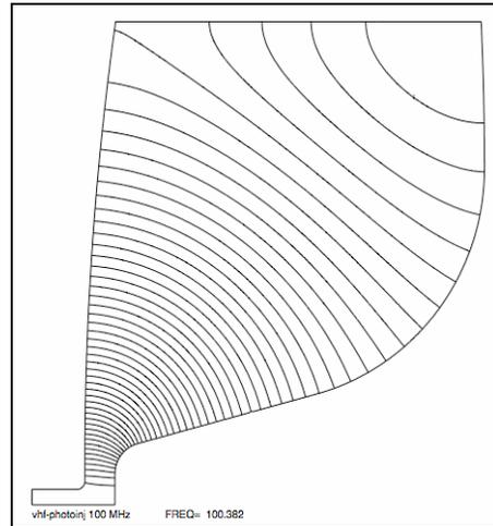
Figure 9: 100MHz cavity geometry.
