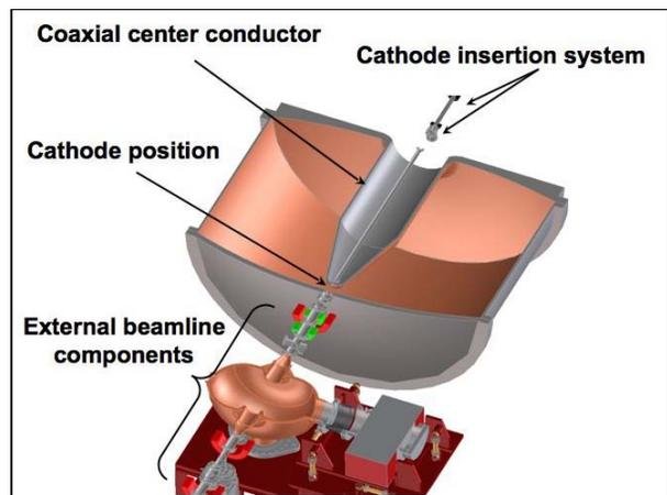
Figure 1: Schematic of a quarter-wave coaxial VHF gun.
