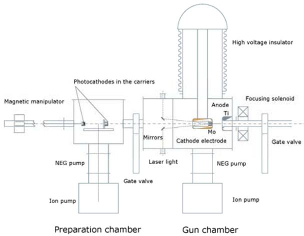
Figure 5. Sketch of the DC photocathode gun.
