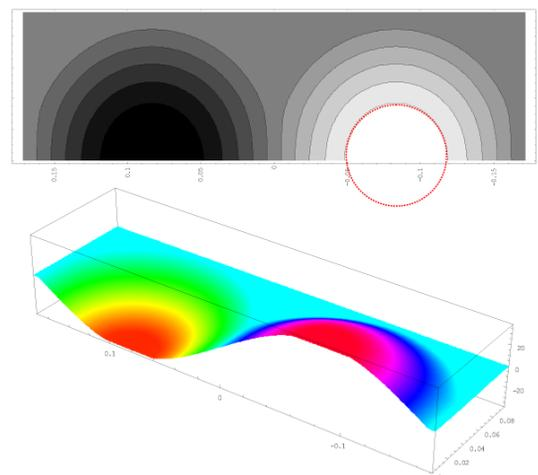
Fig. 6: Contour plot of the integrated accelerating voltage.
