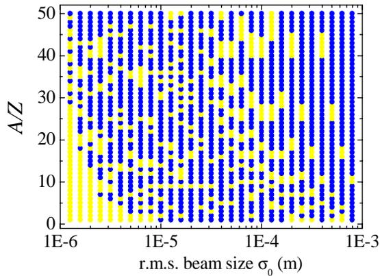
Figure 6: Stability of ion motions under the beam-size modulation. Assumed beam-size ratio ( $\sigma_m/\sigma_0$ ) of 2, the time ratio ( $T_g/T_p$ ) of 10%, a repetition frequency of 2 MHz, and a beam current of 100 mA.
