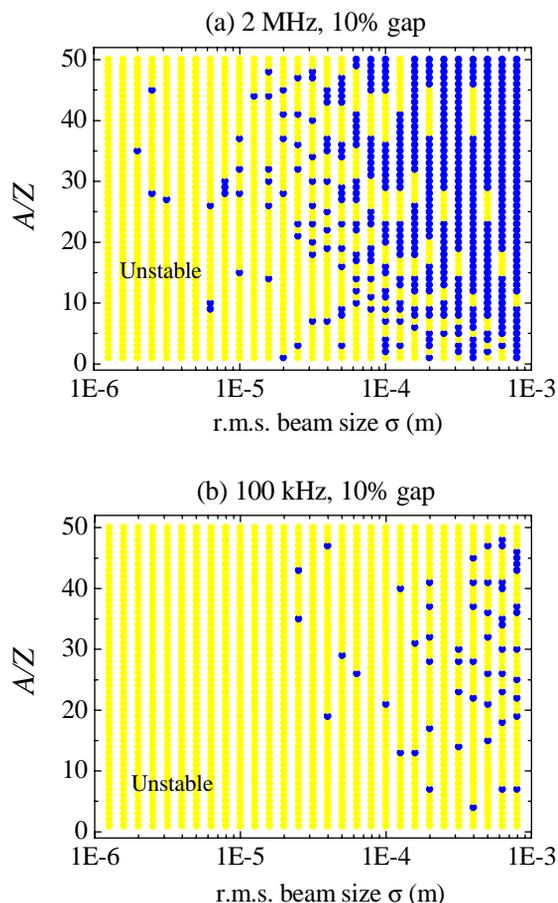
Figure 2: Stability of the ion motions under the bunch gaps. Blue and yellow dots indicate stable and unstable conditions, respectively. Abscissa: beam size (r.m.s.), ordinate: mass number ( $A$ ) per charge number ( $Z$ ) of ions. Assumed 10% ratio of the gap, bunch charges of 77 pC/bunch, and equal beam sizes for the horizontal and the vertical distributions. Repetition frequencies of the gaps are: (a) 2 MHz, and (b) 100 kHz.
