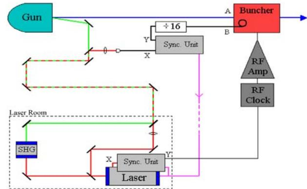
Figure 4: Local and remote synchronisation layouts.
