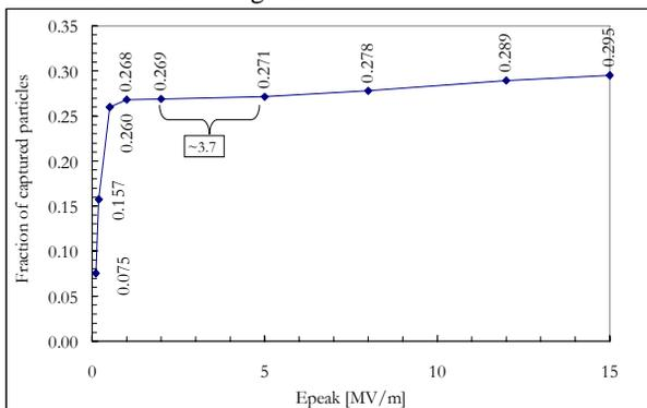
Figure 4: Fraction of photoelectrons which escape the cavity
