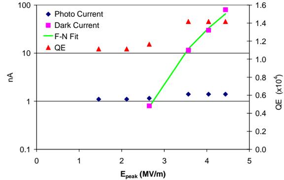
Figure 5: QE for hybrid Pb/Nb cavity
