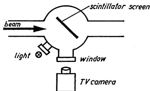
Figure 1: Typical arrangement for observation of beam position and size with a scintillator screen and a TV camera (from [1]).
