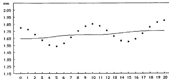
Figure 5: Schematic presentation of beam size evolution over 20 turns, as seen by a screen (OTR or scintillator) or a SEM-grid (from [17]).
