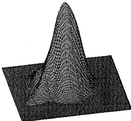
Figure 2: 2-dimensional beam density distribution derived from the light-spot on a scintillator screen (from [3]).
