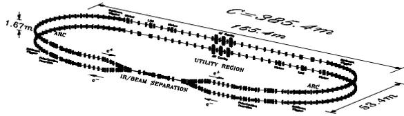
Figure 6: Schematic diagram of the BTCF storage ring
