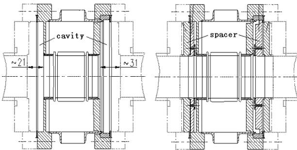
Figure 2: Flanges in BEPC before and after shielding.
