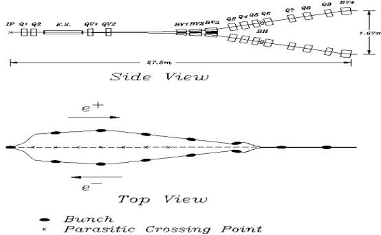
Figure 7: Beam separation and crossing angle scheme.
