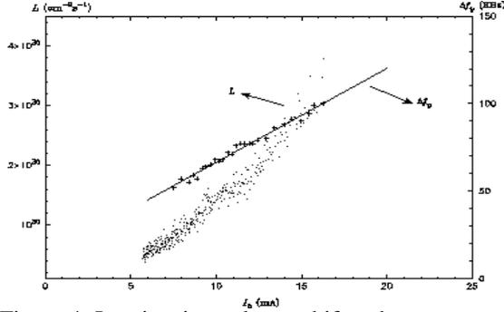
Figure 4: Luminosity and tune shift vs beam current.
