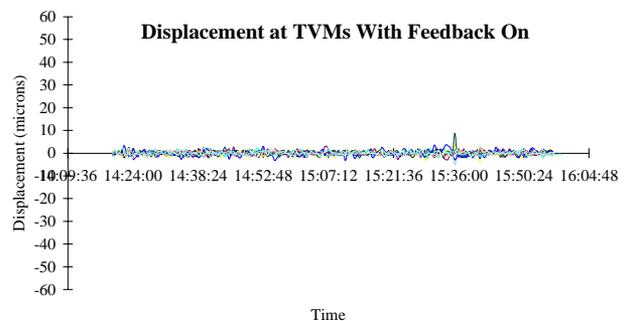
Figure 3: Operation of global vertical feedback on the photon beam monitors during a user beam.
