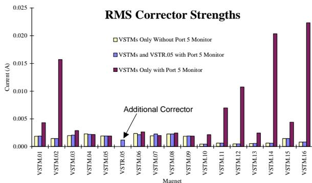
Figure 5: RMS corrector strengths required to correct the orbit at the TVMs with and without dipole 5 TVM.
