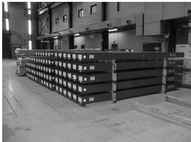
Figure 8: Recycler magnets stacked up and awaiting installation.
