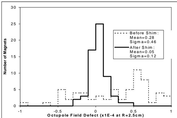
Fig. 6 - Effect of end shimming on the octupole error distribution for Recycler Gradient magnets. Random and systematic defects are at the  $10^{-5}$  level ( $R=2.5\text{cm}$ ) and are about 10x better than typical superconducting magnets.
