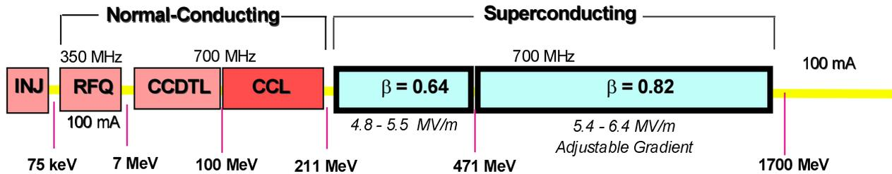
Figure 3 : APT layout for a 3-kg/yr production rate (Linac length = 1220 m)
