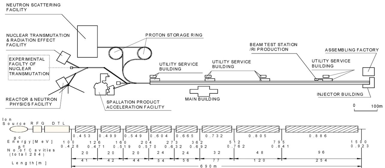
Figure 4 : Layout of the JAERI Neutron Science Project (top) and 1.5 GeV linac design (bottom) (from [11])
