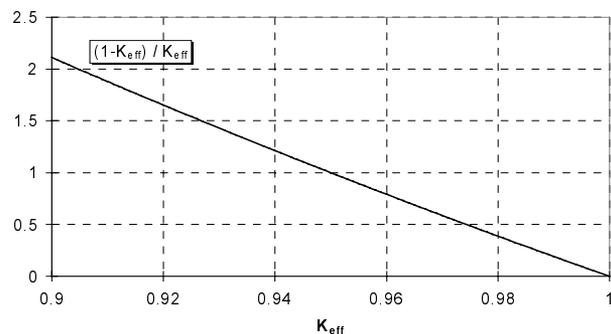
Figure 2 : Beam power evolution with  $k_{\text{eff}}$  (normalized to 1 for  $k_{\text{eff}} = .95$ )
