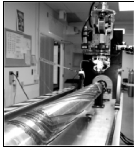
Figure 3: RHIC Helical Magnet Winding Machine.
