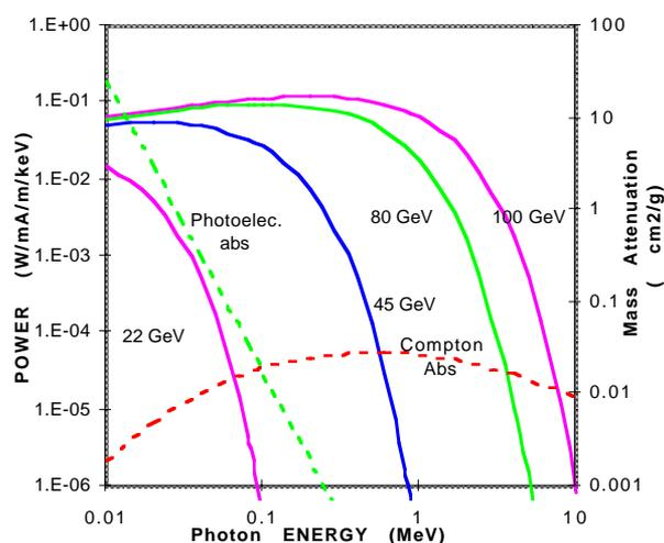
Figure 1: Synchrotron radiation spectrum at various beam energies
