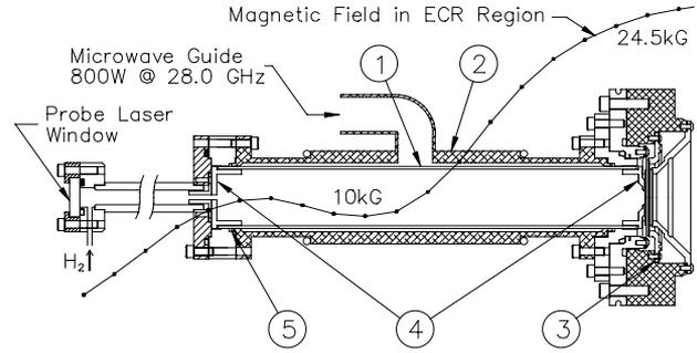
Figure 1: Schematic of ECR proton source; (1) quartz tube; (2) ECR cavity; (3) three plate extraction electrodes; (4) boron nitride end cups; (5) indium seal.
