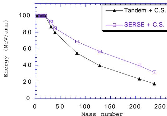
Fig. 5 - The maximum beam energy of the LNS Superconducting Cyclotron.
