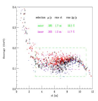
Figure 2: Kinetic energy vs. ct of muons at end of phase rotation channel. The symbols +, o and – denote muons with polarization  $P > \frac{1}{3}$ ,  $-\frac{1}{3} < P < \frac{1}{3}$  and  $P < -\frac{1}{3}$ , respectively.
