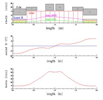
Figure 3: a) Cross section of one cell (2 m) of an alternating solenoid cooling system; b) axial magnetic field *vs.* z; c) beta function *vs.* z.
