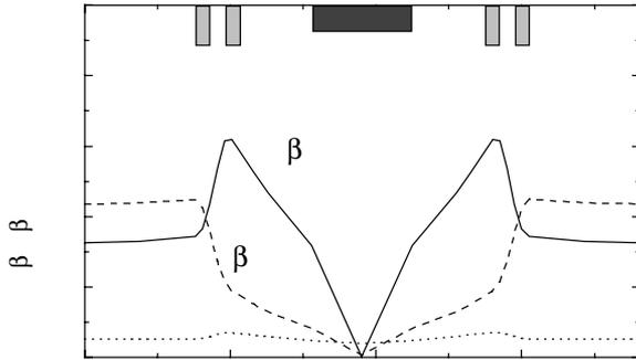
Figure 2: Lattice functions of ELISA for half the circumference.
