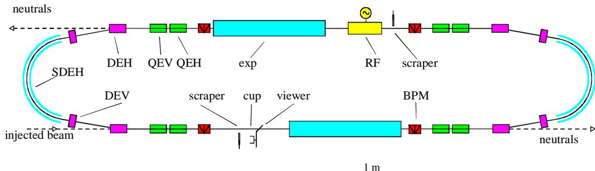
Figure 1: Layout of the ELISA storage ring. The abbreviations are explained in the text.
