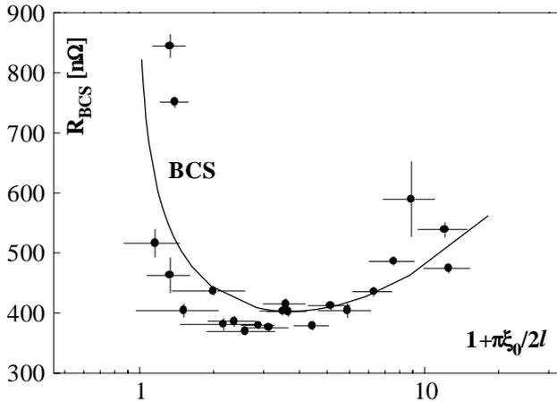
Figure 3. The BCS resistance at  $T=4.2\text{K}$ .
