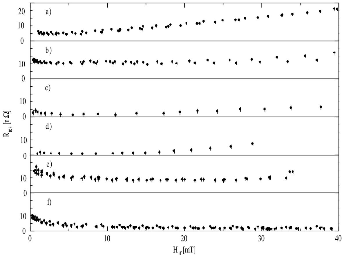
Figure 9. Residual resistances of film (a to d) and bulk (e to f) cavities.
