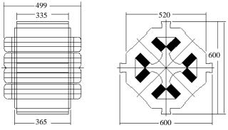
Figure 2: General layout of the quadrupole magnet
