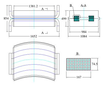
Figure 1: Technical design of the dipole magnet
