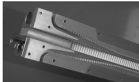
Figure 7: A four-channel decelerator structure.
