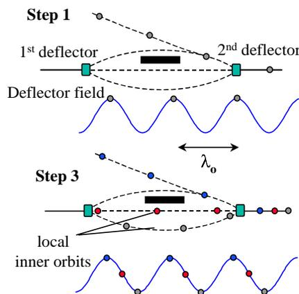
Figure 2: Injection region in the times-four combiner.
