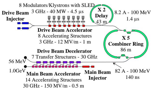
Figure 9: A Two-Beam Accelerator test facility
