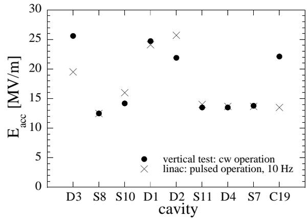
Figure 4: Performance of cavities in the linac compared to vertical test results.
