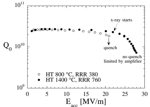
Figure 1: Improvement of cavity C21 after a 1400 °C heat-treatment.
