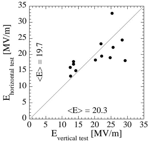
Figure 2: Comparison of horizontal (pulsed mode) and vertical (cw mode) tests.
