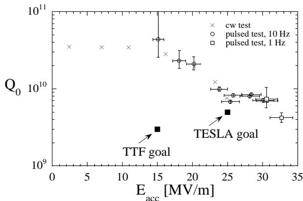
Figure 3: Horizontal test result of cavity C23 compared to vertical test.
