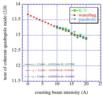
Figure 3: Coherent quadrupole tune vs. intensity. The tune shift is independent of the initial distribution for equivalent beams.
