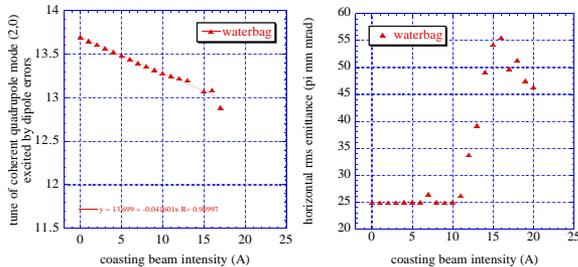
Figure 8: When a C.O.D. exists, a coherent mode resonates with image charge and emittance growth occurs.
