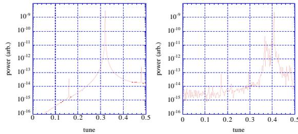
Figure 2: Spectrum of coherent quadrupole mode with zero intensity (left) and at 2A (right). The peak in the left corresponds to the tune of 13.68 (twice of the bare tune). A move towards the right means decreasing of tune.
