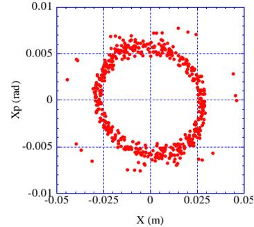
Figure 9: Halo particle found in the multi-particle tracking. Parametric resonance excited by coherent quadrupole mode is the source of halo formation. Resonance structure is clearly seen.
