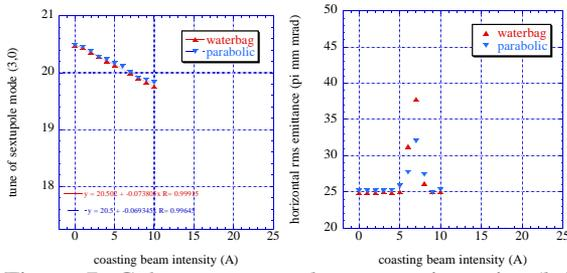
Figure 7: Coherent sextupole tune vs intensity (left) and rms emittance vs intensity (right). One peak of the tune corresponds to almost three times of the bare tune is depicted. The rms emittance growth occurs when the coherent sextupole tune hits an integer.
