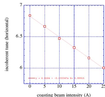
Figure 1: Incoherent tune shift vs. beam intensity.
