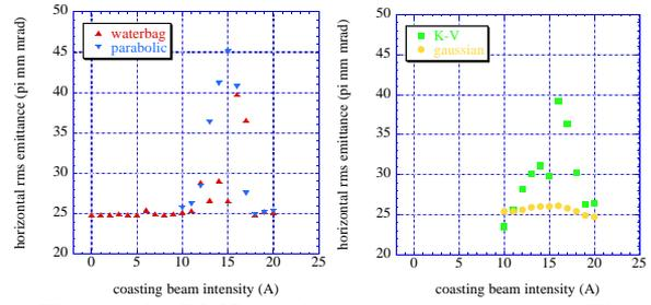
Figure 4: RMS emittance vs intensity. The rms emittance growth occurs when the coherent quadrupole tune hits an integer.
