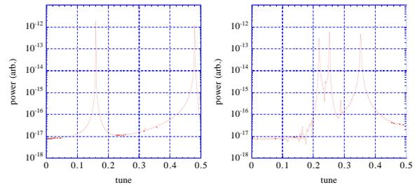
Figure 5: Spectrum of coherent sextupole mode with zero intensity (left) and at 2A (right). In the left figure, a peak on the left corresponds to the tune of 6.84 (same as the bare tune). A peak on the right does 20.52 (three times of the bare tune). The left peak splits into two when the intensity is increased.
