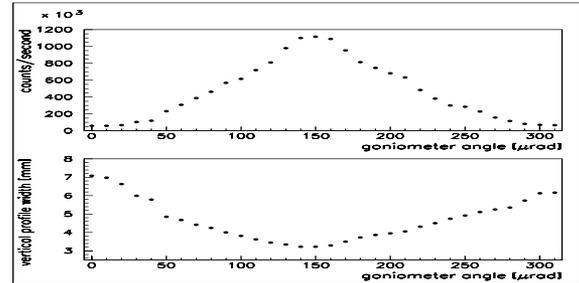
Figure 2: Angular scan and width of vertical profiles
