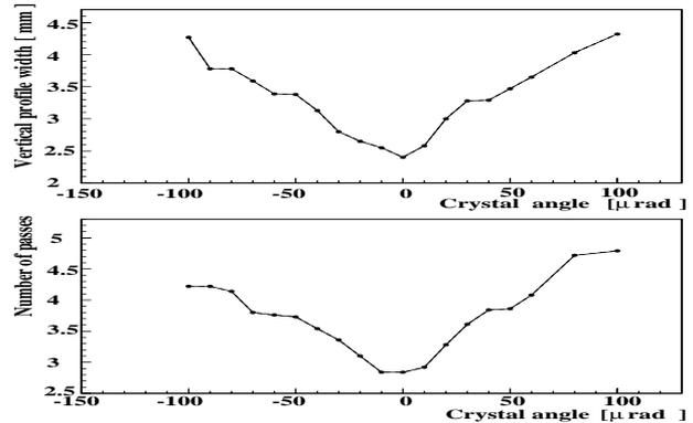
Figure 3: Simulated vertical width and number of passes
