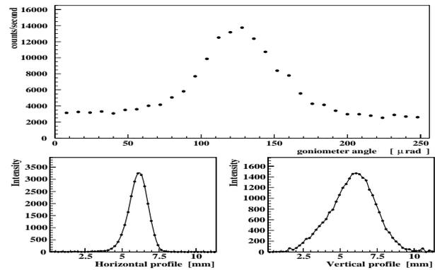
Figure 5: Angular scan and profiles obtained with Pb ions
