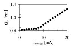
Figure 6. Bunch lengthening for 3.4 MV
