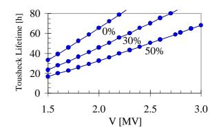
Figure 3. Touschek lifetime as a function of RF voltage for the three multibunch modes.
