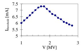
Figure 2 Bunch current threshold as a function of voltage.
