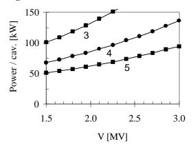
Figure 4. Power per cavity as a function voltage and number of cavities, for 250 mA beam.
