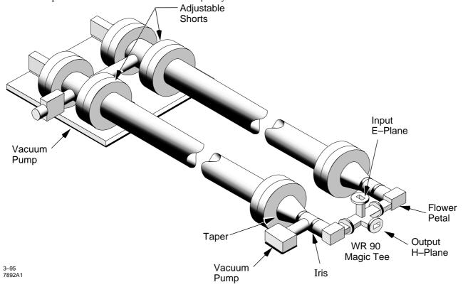
Figure 1. SLED-II Layout. It has two 12.065 cm diameter waveguide, 35.35 m in length (223 nS round-trip time.)
