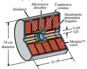
**FIGURE 3.** A proposed RK-TBA induction cell design illustrating longitudinal core segmentation.
