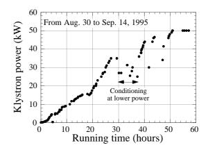
Fig. 2. Progress of the conditioning. The output power of the klystron is plotted against the net conditioned time. Note that the input power of the cavity was about 2% lower than the klystron power, due to the insertion loss of the circulator.
