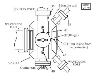
Fig. 3. Measured temperatures (°C) of the cavity under an input power of 50 kW. Input water temperature,  $31^{\circ}$ C.
