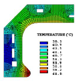
Fig. 4. Result of a thermal analysis on the axisymmetrical cavity model using the ANSYS code. Assumed a dissipated power of 50 kW/cavity, water temperature of 30°C and a heat-transfer coefficient of 1.2  $W/cm^2/K$  on the cooling channels.
