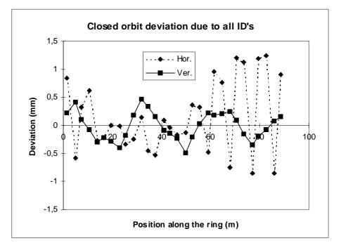
Figure 1. Closed orbit deviation with all ID's closed.
