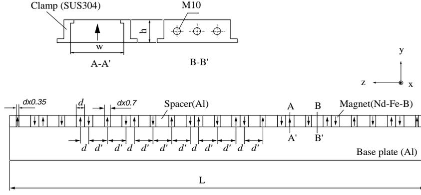
Figure 1 Magnetic structure of the quasi-periodic undulator
