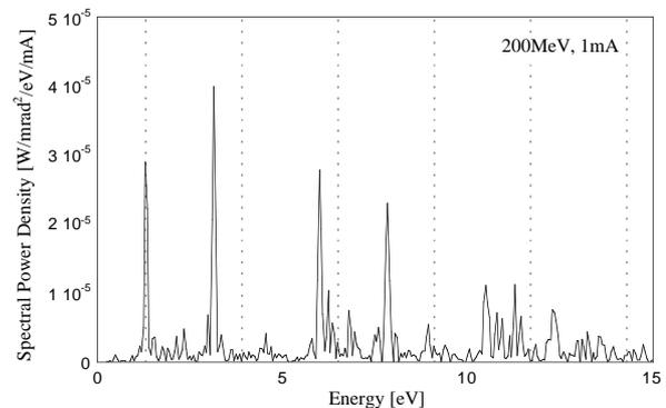
Figure 6 The radiation spectrum calculated from measured field data. gap=36mm
