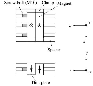
Figure 2 Magnetic field correction structure
