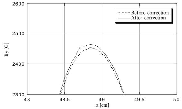
Figure 3 Magnetic field correction by a thin plate. Thickness of plate is 0.05mm. gap=36mm
