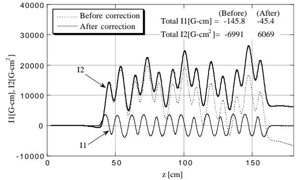
Figure 5 The 1st-integral(I1) and 2nd-integral(I2) distributions at gap=36mm.
