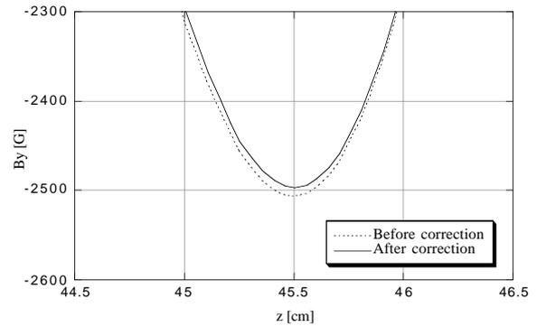
Figure 4 Magnetic field correction by flux shunt. gap=36mm
