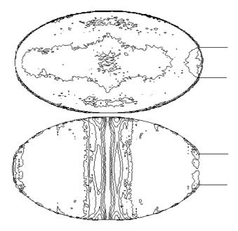
Fig. 1. Contour level plots of the electron cloud. Top: pumping straight section. Bottom: dipole bending magnet. The beam orbit is at the center of the ellipse. The antechamber slot is shown at the right-side of the chamber. The ratio between successive levels is 2, and the top level is at 99% of the peak.
