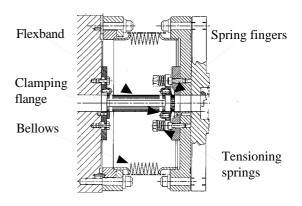
Figure 1. Bellows assembly showing flexband, tensioning springs, and spring fingers
