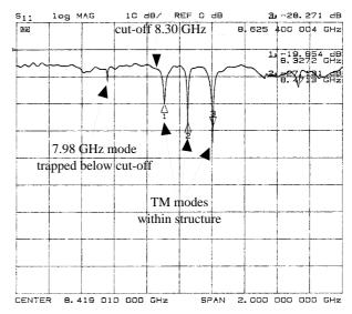
Figure 6. S<sub>11</sub> measurement showing resonances in apparatus and trapped mode localised in flexband
