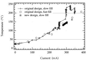
Figure 4. Flexband heating, original (bulging) design and new (straight) design.
