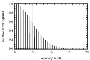
Figure 3. Beam power spectrum 320 bunches, feedback off, bunch length  $\sigma = 24 \text{ ps}$
