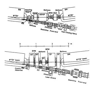
Figure 3. Configuration of present (upper) and new (lower) lattice at a normal cell.
