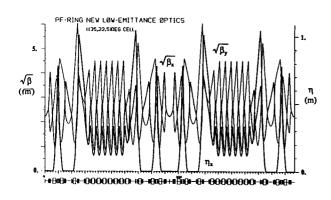
Figure 2-b. Optical functions of the new lattice of the lowest emittance (27 nm-rad). The whole ring is shown.
