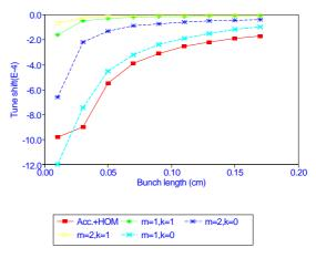
Figure: 4 Tune shift and bunch length for the several modes.
