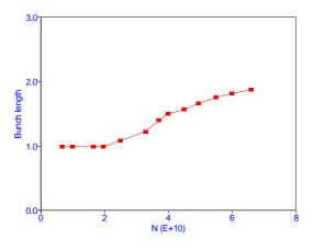
Figure: 1 The bunch length due to the PWD by the simulation method.
