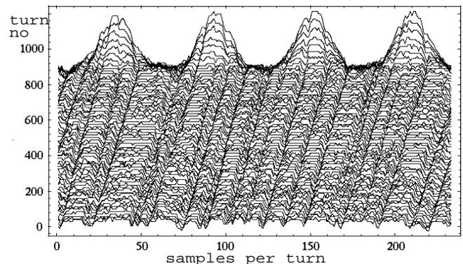
Fig. 1: Longitudinal beam pick-up signal recorded 20ms after multi-turn injection into SIS ( $I_{beam} \approx 5 \text{ mA}$ ). Each trace corresponds to the longitudinal beam density over one turn.
