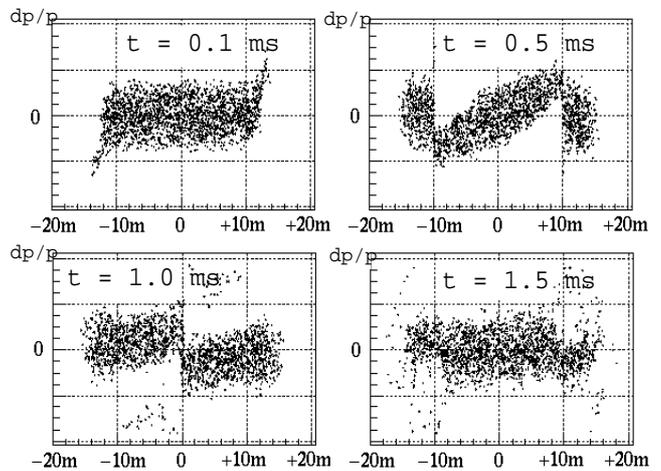
Fig. 6: Computer simulation of the longitudinal phase space distribution (momentum vs. location) after multi-turn injection. A small number of particles are not captured inside the barrier bucket and will be lost later.
