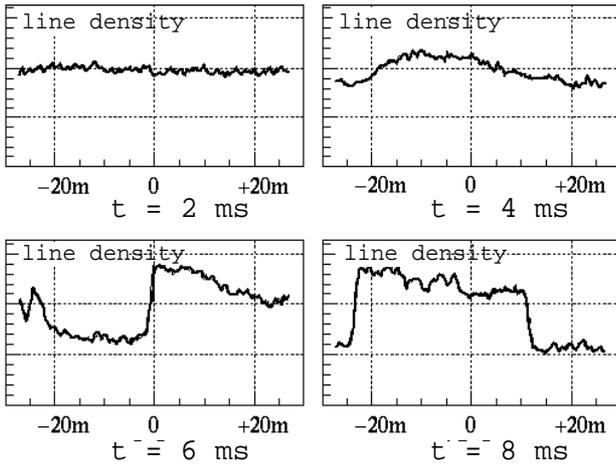
Fig. 2: Computer simulation of a longitudinal beam signal (line charge density over 1/4 of the machine length) with respect to space charge and strong beam -RF cavity interaction.
