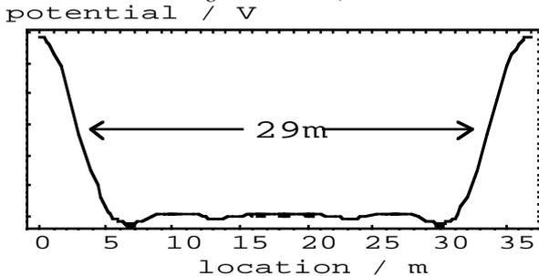
Fig. 5: Potential using 5 Fourier harmonics according to the parameters of fig. 4. Note the small waviness (<5%) at the bottom of the potential.
