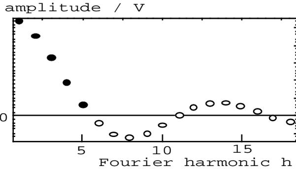
Fig. 4: Fourier coefficients of a rectangular barrier bucket up to the 18th harmonic of the RF fundamental frequency (bunch length = 25m, bucket length = 29m, RF fundamental wave length = 36.65m).
