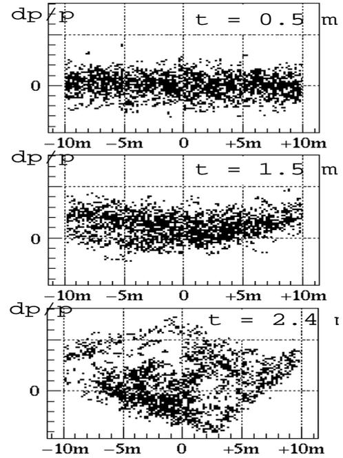
Fig. 3: Computer simulation of the development of the longitudinal phase space (particle momentum vs. longitudinal location) due to beam-cavity interaction with respect to space charge effects in a HIDIF accelerator.
