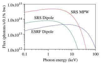
Figure 3. Comparison of photon fluxes from the SRS and ESRF dipoles and the proposed MPW.
