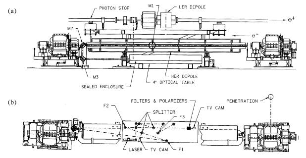
Figure 1. HER and LER beamlines in the middle of Arc 7 in (a) an elevation view and (b) a plan view, showing path of the synchrotron light. For clarity, only the HER optics are shown in the sealed optics chamber below the HER dipole.
