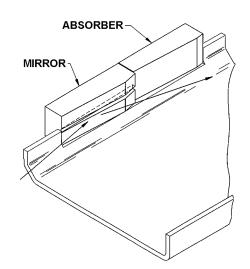
Figure 2. The slotted first mirror and the x-ray absorber, both mounted in the HER chamber wall.
