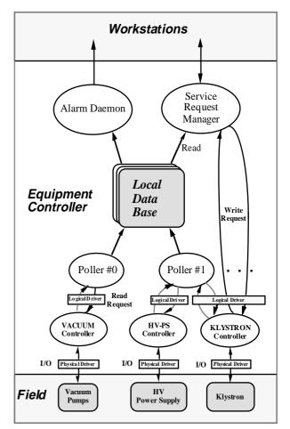
Figure 2: The low level software framework.
