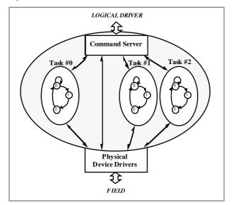
Figure 3: Device Controller structure.
