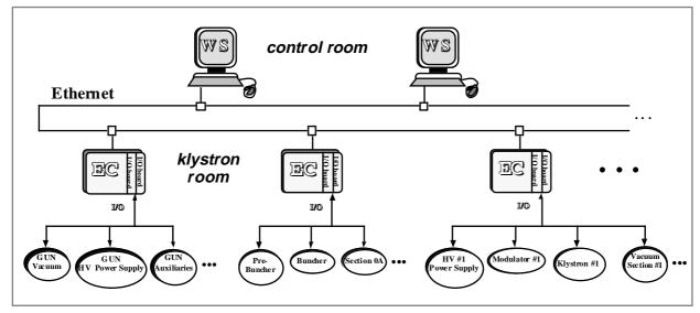
Figure 1: Linac control system architecture.
