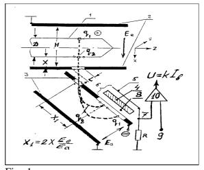
Fig. 1 Simplified scheme of the beam crossection ionisation detector. 1 - the beam under investigation; 2 - extractor; 3 - analysator; 4 - MCP; 5 - scinscilating screen; 6 - opened ICT; 7-output signal for the beam current monitoring; 8 - additional accelerating interval; 9 - corrective signal; 10 - regulated amplifier
