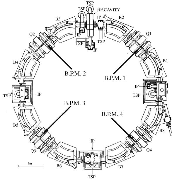
Figure 1 : Plan view of SOR-RING.
