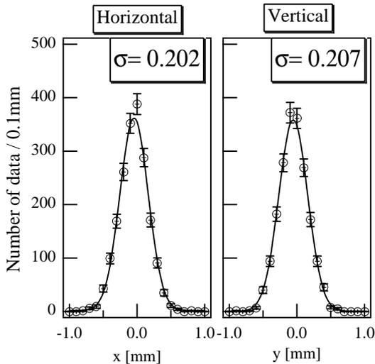
Figure 6 : Relative accuracy of the single-pass monitor system. The total number of data is 1000.
