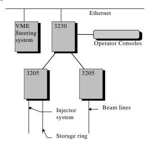
Figure 2: SRS Control System in 1993
