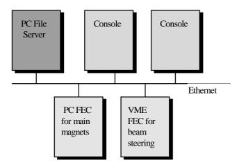
Figure 3: The Upgrade Control System
