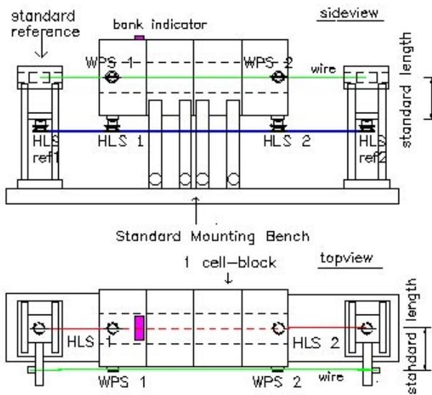
figure 4: cell-block alignment on the bench
