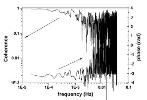
Figure 4: Coherence and phase difference obtained in the welded tuff tunnel. Two levels were set up 46 meters apart.
