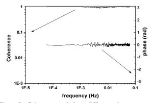
Figure 2: Coherence and phase difference between two sensors separated by 50 cm with no expansion joint.
