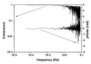
Figure 5: Coherence and phase difference obtained in the granite tunnel. Two levels were set up 46 meters apart.
