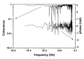
Figure 3: Coherence and phase difference between two sensors separated by 50 cm with an expansion joint.
