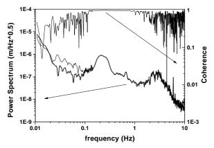
Figure 1: A typical example of the ground vibration in KEK. The spectra were observed by two seismometers at a distance of 48 meters.
