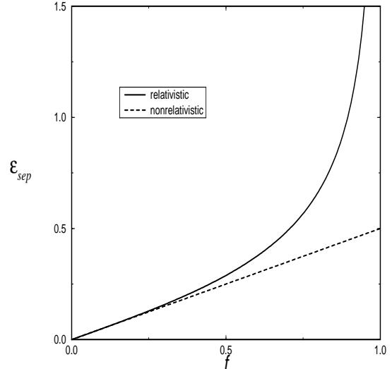
Figure 2: Wave amplitude  $\epsilon_{sep}$  vs. the normalized wave phase-velocity  $f$ . Solid (dashed) line represents the relativistic (nonrelativistic) case.
