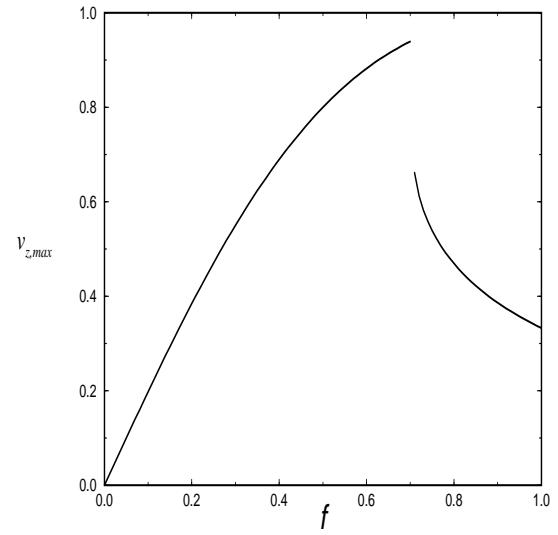
Figure 3: Maximum fully relativistic longitudinal speed  $v_{z,max}$  vs.  $f$  for  $\epsilon = 0.5$ .
