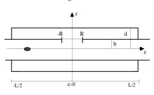
Figure 2 : Coaxial resonator.
