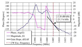
Figure 1: Longitudinal BTF measured in the PSB
