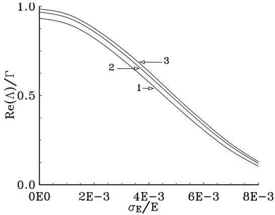
Figure 4: Dependency of the FEL amplifier field gain on energy spread: (1) -  $2 \times 0.25$  TeV variant; (2) -  $2 \times 0.5$  TeV variant; (3) -  $2 \times 1$  TeV variant.
