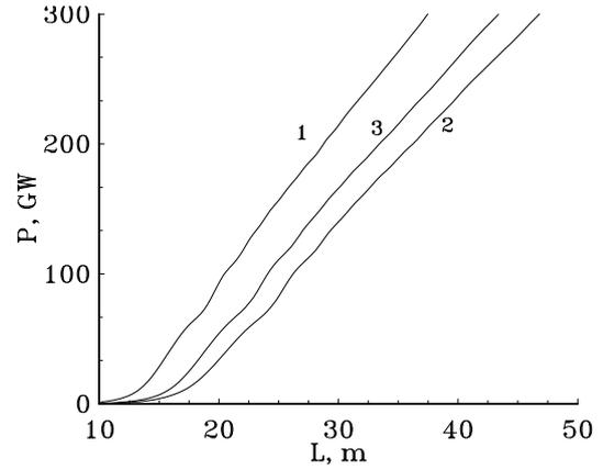
Figure 5: Output FEL amplifier power versus undulator length: (1) -  $2 \times 0.25$  TeV variant; (2) -  $2 \times 0.5$  TeV variant; (3) -  $2 \times 1$  TeV variant.
