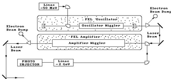
Figure 2: Two-stage FEL scheme for a photon collider.
