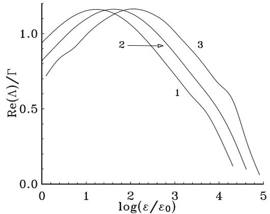
Figure 3: Dependency of the FEL amplifier field gain on emittance ( $\epsilon_0 = 10^{-6} \text{cm} \times \text{rad}$ ): (1) -  $2 \times 0.25$  TeV variant; (2) -  $2 \times 0.5$  TeV variant; (3) -  $2 \times 1$  TeV variant.
