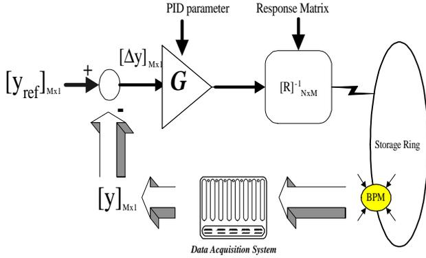
Figure 1: Block diagram of digital global feedback.
