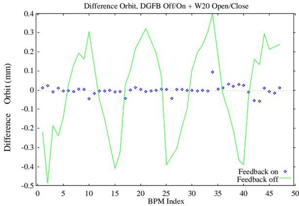
Figure 3: Difference orbit between wiggler open and close with feedback on/off.
