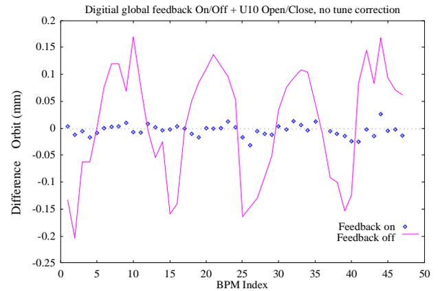
Figure 2: Difference orbit between undulator open and close with feedback on/off.
