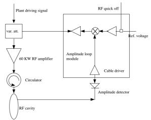
Fig. 2 Simplified block diagram of the amplitude loop
