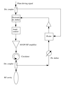
Fig. 3 Simplified block diagram of the phase loop
