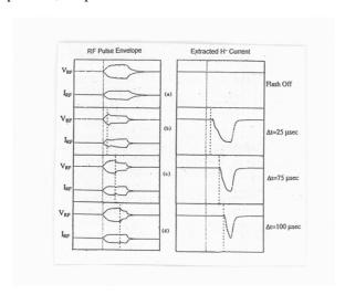
Fig. 4 Oscilloscope trace showing the modulated H<sup>-</sup> ion beam current when a positive voltage pulse is applied on the plasma electrode.
