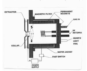
Fig. 1 Schematic of the rf-driven multicusp H<sup>-</sup> ion source.
