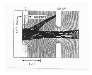
Fig. 3 Planar calculation showing the effect on the extracted electrons due to a pair of permanent-magnets located inside the first electrode.
